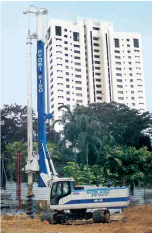
BANGLADESH E6050-SM240 e E6050LM-SM240 pali Soil Mixing.
